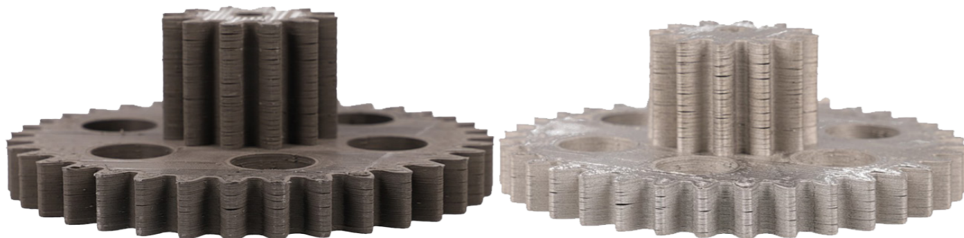
Figure 6: Print Delamination Become Sintered Cracks
