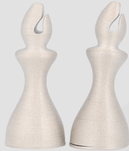
Figure 14: Warped Bottom Can Lead to Failure
